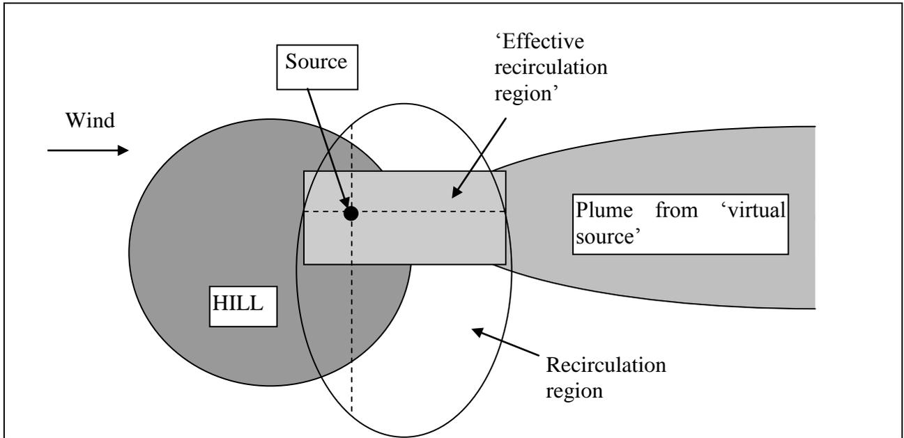
**Figure 4.1** The recirculating region and effective recirculating region
