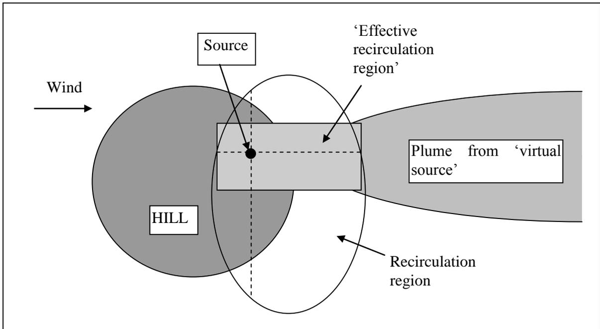
**Figure C.1** The recirculating region and effective recirculating region
