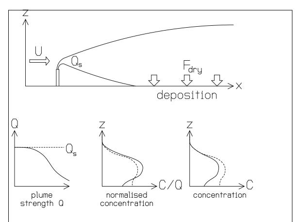
**Figure 1**: Effect of dry deposition on vertical concentration profile. In the lower 3 figures the dashed line represents the case without dry deposition and the solid line the case with dry deposition.
