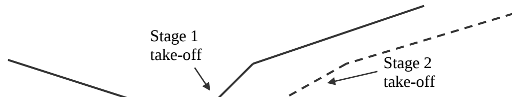
Figure 4.3 – Example trajectories for aircraft with different weights
